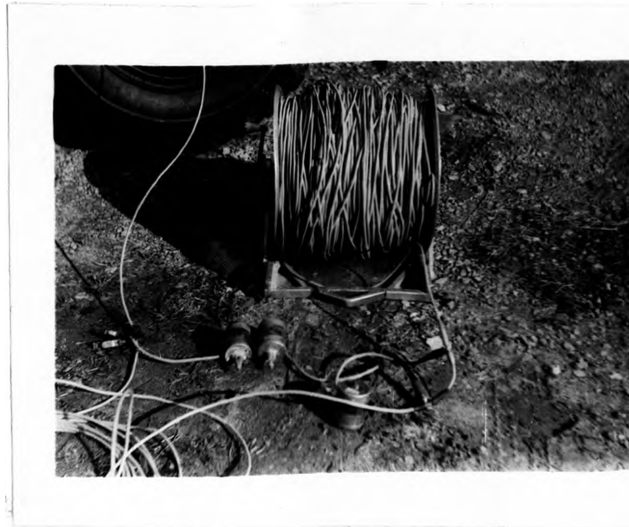
a. Breast reel, geophone cable and geophones. A single geophone is shown attached to cable.
